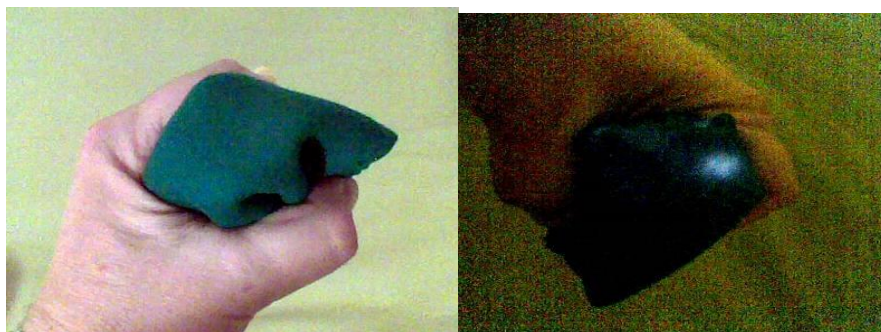
Fig. 12a and 12b: Felt completely blocks visible light but not infrared.
